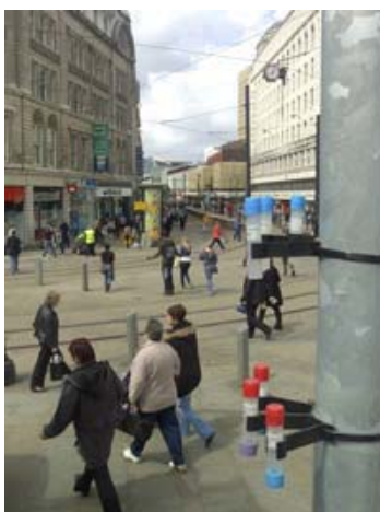
Urban air quality measurements taken via test tubes mounted to utility poles
